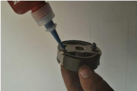
Place the pins on both sides, also place the washers and nuts put a loctite handle to block the threads.
