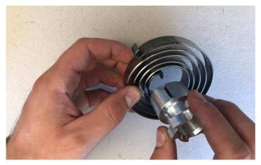
Grease the spring carefully. Couple the serrated pin with the spring, fitting the latter in the specific slot.
