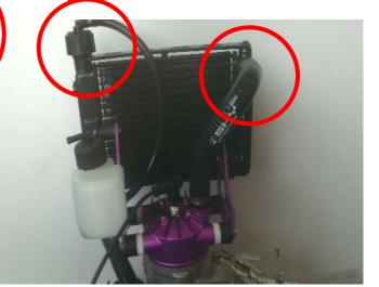
Check the fitting positions and insert the clamp straps as in the photos.
