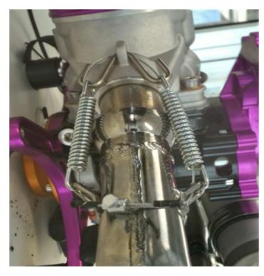
Finally, insert the steel cable between the hooks by sliding it into the springs and tie it to the manifold side as in the picture below.
