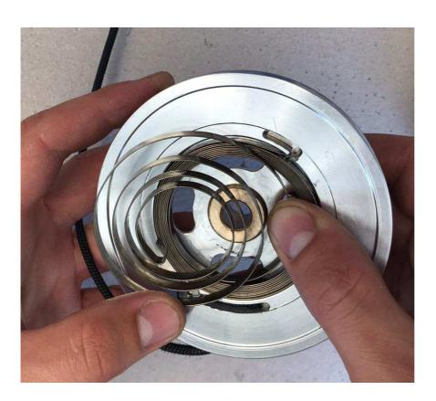
Insert the cord in the hole of the pawl; tighten the grub screw on the cord, then insert it in the hole of the pulley. Lastly, fit the pawl in the specific hole on the pulley and wind the cord 8 rotations in the pulley as shown in the figures.
