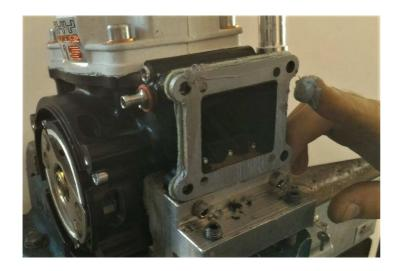
Place another r layer of motorsil on the outside of the glue box, another paper gasket, and still motorsil, finally installing the carburetor and tightening as shown in the following figures.
