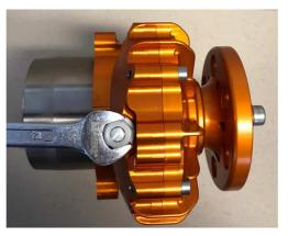
If you have a finned reduction, unscrew the cap located in the upper rear part and insert 60 ml of synthetic transmission oil.
