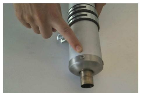
Unhook the tube base and remove the tube by holding the silencer out of the socket; then remove the worn glass wool.
