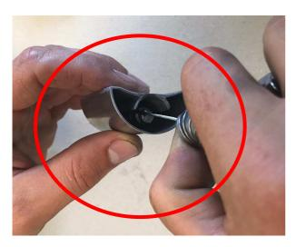
Proceed to replace the cable, ensuring you have correctly fitted the end of the cable in the compartment of the guillotine as displayed in the figure below.
