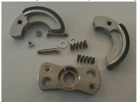
Place the spring in the seat of the pile and place the clutch body as shown in the figure. Do this also on the other side.
