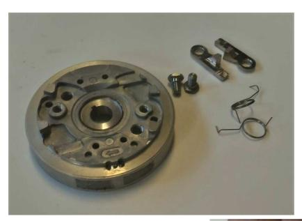
Position the spring in the specific hole and in the flywheel guide as in the photo to the side.
