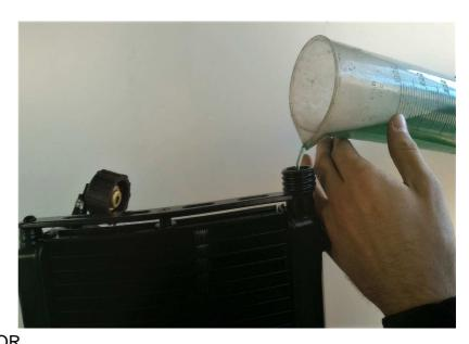
THE EXCESS LIQUID IN THE TANK MAY FLOW OUT AND IF LEAKS ARE NOTED, FIRSTLY CHECK THIS; IT MUST NOT EXCEED THE LEVEL INDICATED.
