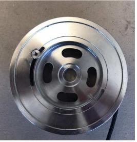
Position the rope in the specific hole of the cup. Insert the ignition unit assembled in the cup and connect the end of the small spring to the cup.
