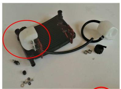
Place the radiator on the cover and put the tubes to their respective outlets as shown below.
