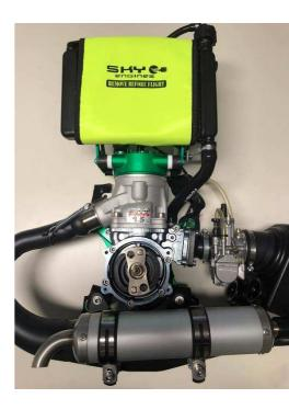
Unscrew the cap of the reduction unit and proceed to change the oil after 30 hours of use. Having accurately emptied the reduction body of consumed oil, proceed to replace with new oil.
