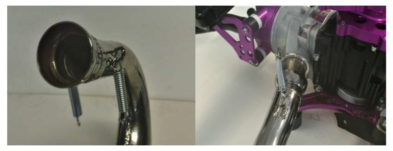
Tighten with 2 screws M6 x 12 and washers the muffler fittings with silent blocks of the engine chassis;
