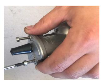
Open the cap by removing the spring and the guillotine. Hold the spring as in the figure, releasing the cable from its compartment in the guillotine.
