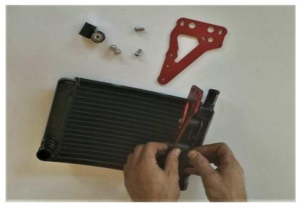
Mount the special silent blocks on the radiator and then the brackets on the silent blocks (on both sides)
