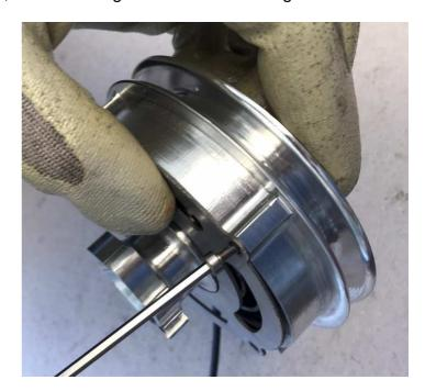
Insert the small spring from the other side of the pulley. As before, fit the spring well in the specific compartment.
