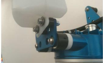
Finally mount the radiator on the silent blocks.
