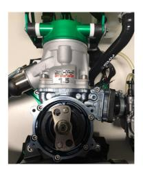
Tighten the nut without tightening the clutch body completely, leaving the relatively free mops in the picture.
