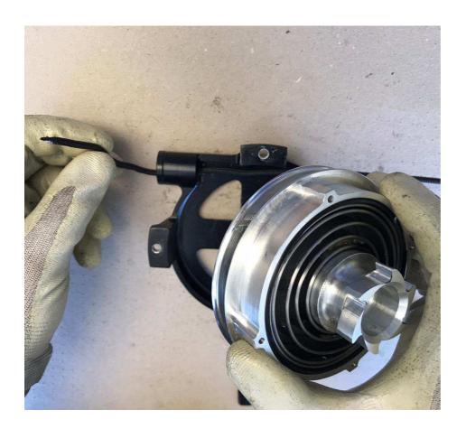
Insert the bushing as in the figure and tighten it to the serrated pin.
