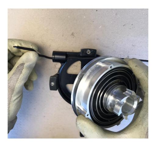
Insert the bushing as in the figure and tighten it to the serrated pin.
