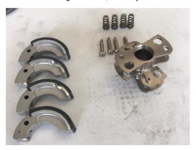
Position the spring in the specific compartment of the shoe and position the clutch body as demonstrated in the figures.
