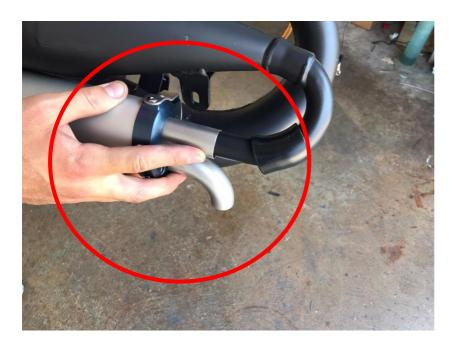
Screw in the silencer on the specific hooks on the exhausts, without forgetting the aluminium shim.
