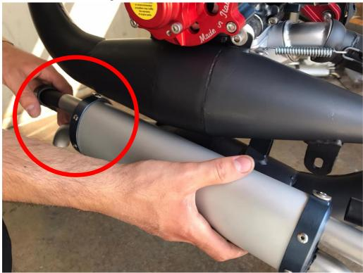
Then, insert the silencer on the manifold of the upper exhaust as in the figure.
