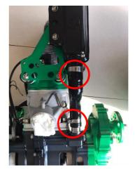
Check the positions of the joints and insert the tube tightening clamps as in the photo.
