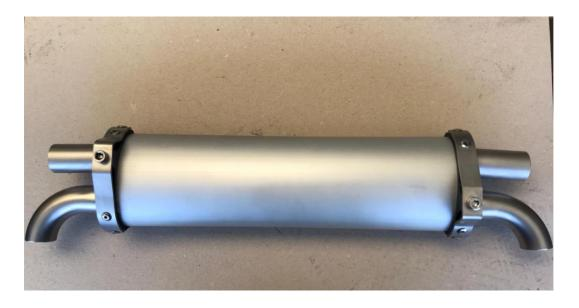
Before inserting the silencer, ensure you have positioned the rubber sections on the manifolds of the exhausts, as the first operation
