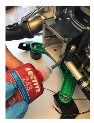
Place a drop of red Loctite in the holes for the screws
