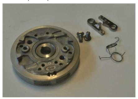
Position the spring in the specific hole and in the flywheel guide as in the photo to the side.
