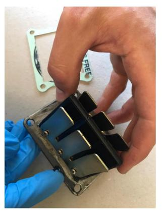
Apply and evenly distribute a non-excessive quantity of Motorsil on the internal flange, avoiding dripping along the entire duct. Position the specific "paper" gasket and distribute another layer of Motorsil the same as the first as in the following figures.
