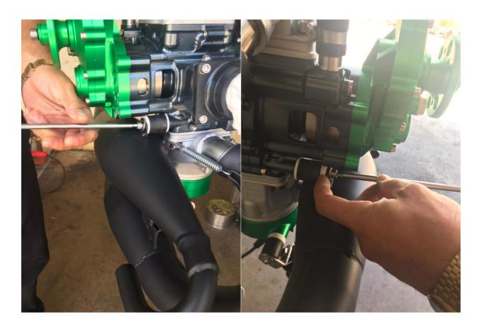
Repeat the same procedure for the lower exhaust. Lastly, for the lower exhaust, adjust the correct inclination by tightening the screw as circled in the image below.
