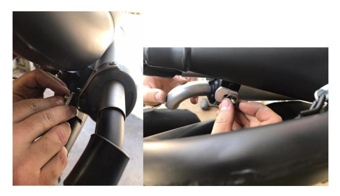
Slide the rubber sections to totally cover the slot between the silencer and the manifold of the exhaust.
