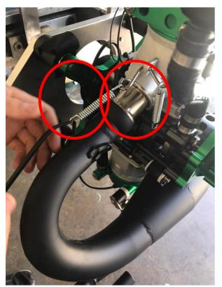
Insert the manifold of the upper exhaust in the respective receptacle of the upper cylinder.
