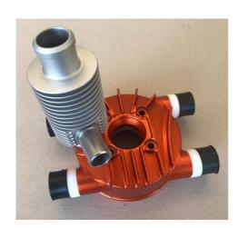
Assemble the Teflon disc and then the silent block on the upper head cover as in the figure to the side. Then, assemble the head cover dissipator.
