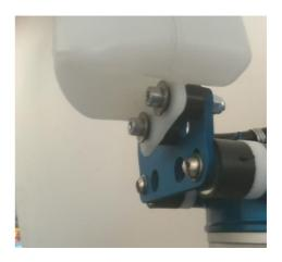
Lastly, assemble the radiator on the specific silent blocks.
