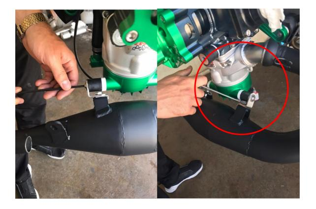
Lastly, insert the steel cable between the hooks, letting it pass inside the springs and tie it to the side of the manifold as in the figure below.
